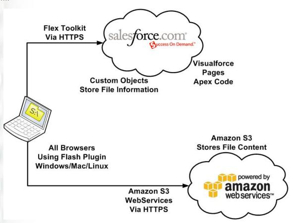
The following sections describe the individual components used in the above architecture diagram and explain the security features of each component.
